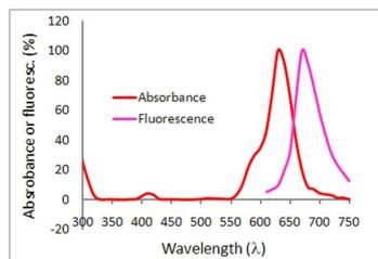
**Figure 3. Spectral Scans of HiLyte Fluor™ 647 labeled tubulin protein.** Labeled tubulin protein was diluted with sterile distilled water and its absorbance and fluorescence spectrum was scanned between 250 and 750 nm. Absorbance peaks at 640 nm and fluorescence at 670nm.
