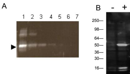
A) Titration of acetylated BSA lanes 1-5 contain 0.5, 0.1, 0.05, 0.01, and 0.005 ng Ac-BSA, lanes 6-7 contain 500 and 1000 ng non-acetylated BSA, respectively. AAC01 recognizes 0.005 ng of chemically acetylated BSA. Arrowhead indicates acetylated BSA, higher molecular weight bands are acetylated BSA oligomers.
